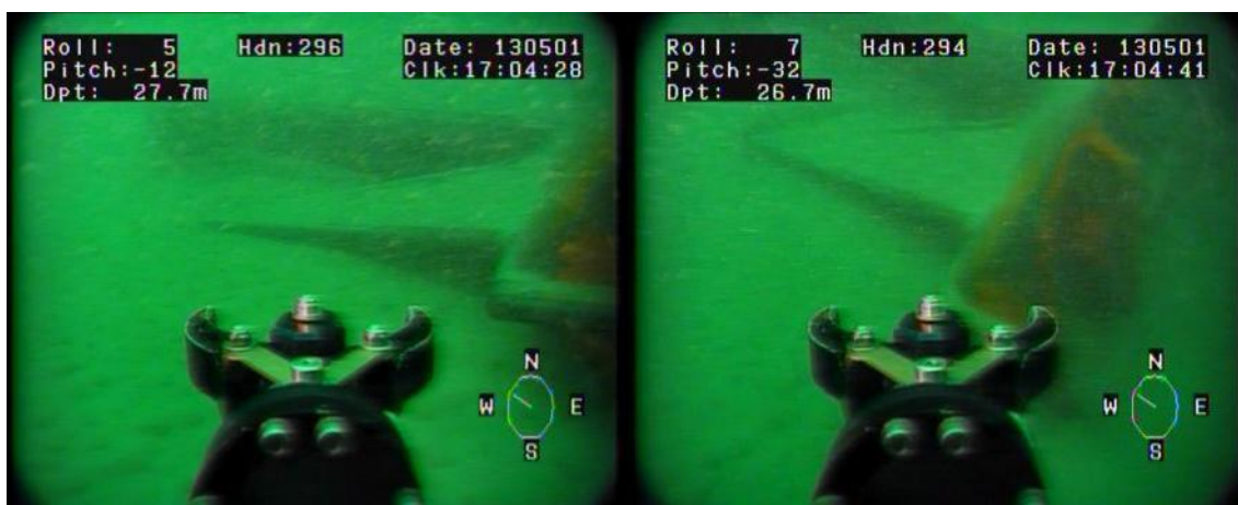
Figure F.3 AC14 at VTG-3 Anchor at rest (left) and tips initial penetration (right)
