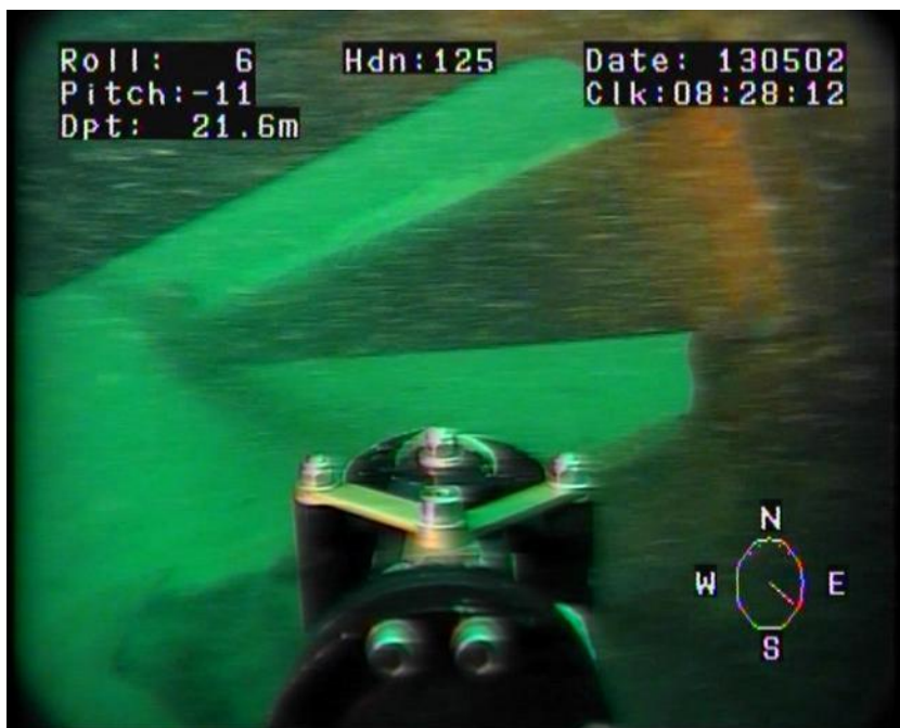
Figure F.9 VTG01_AC14_20130502_08h28m012_Anchor askew broken out.jpg
