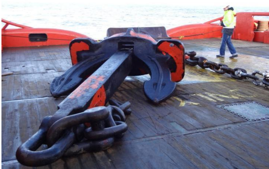
Photo A.1 11.5 t Hall anchor on deck of Esvagt Connector
