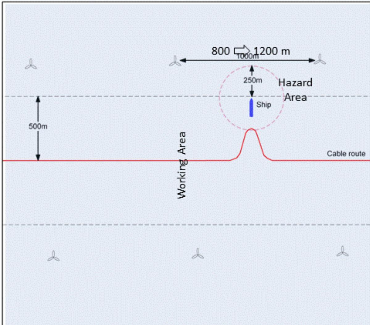
Figure 4 - Vessel operation on the extent of the Working Zone when deploying a final bight
