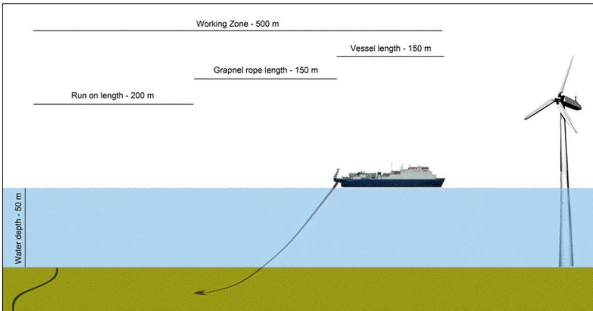
Figure 2 - Indicative distances required within the Working Zone when conducting cable recovery with grapnels in 50m depth of water (ESCA Guideline No 6)
