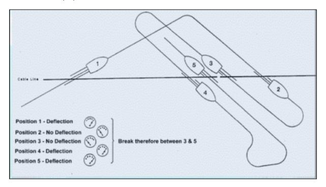
Figure 1 - The process of determining fault location through the use of trailed electrodes. (Internal Document, GMSL, 2011)
