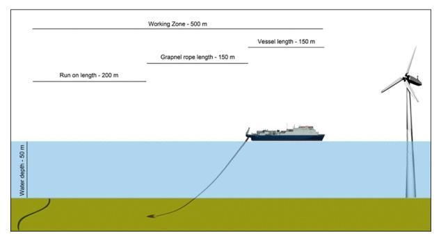
Figure 2 - Indicative distances required within the Working Zone when conducting cable recovery with grapnels in 50m depth of water (ESCA Guideline No 6)
