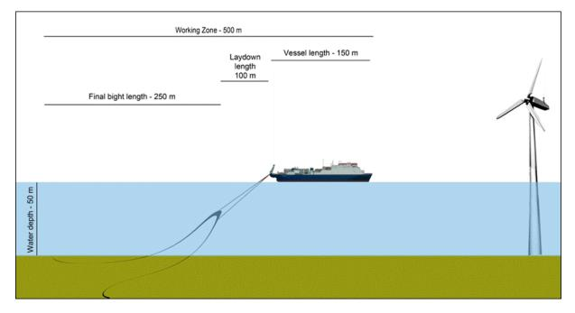
*Figure 3 - Indicative distances of cable line within the Working Zone when deploying a final bight to the seabed in 50m depth of water*
